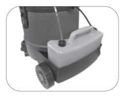
Connect the detergent outlet pipe to the rear of the valeting machine; Line up
