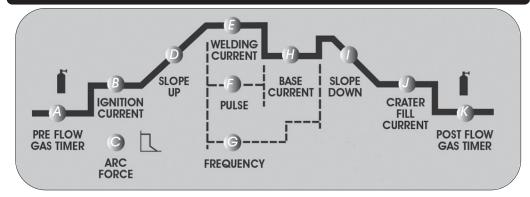
The welding parameters for each mode (where available) are selected by pressing the Parameter Select / Adjust Control, and are adjusted by turning the Parameter Select / Adjust Control. The selected parameter will be displayed when the light is illuminated.
