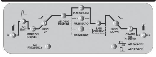
The welding parameters for each mode (where available) are selected by pressing the Parameter Select buttons:
