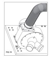
Fit the double inlet adaptor over the inlet on the collector body / motor housing and secure in place with the screw provided. FIG. 10.
