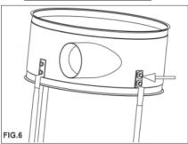
Fit the upper bag support to the 3rd support as shown and fully tighten all bolts to secure. FIG. 7.
