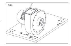
Fit the gasket to the outlet opening of the collector body / motor housing. FIG. 3.
