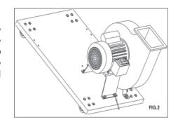
Fit the collector body / motor housing to the motor support bracket as shown, using the bolts, washers and nuts provided. Then fit the whole assembly to the main base using the bolts and washers provided. Fully tighten all nuts / bolts to secure. FIG. 2.
