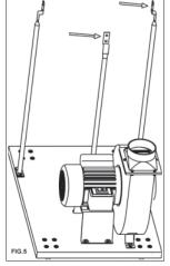
Fit the collector as shown with the bolts and washers provided. **Note:** Only fit the 2 x side supports with bolts at this point; leave the 3rd one free. FIG. 6.
