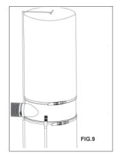
Fit the collection / filter bags over the collector as shown. Secure in place with the bag clamps provided. FIG. 9.
