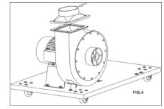
Fit the inlet adaptor over the gasket ensuring that the holes all line up. Secure in place with the bolts, washers and nuts provided. Fully tighten secure in place. FIG. 4.
