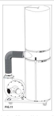
When the dust collector has been fully assembled, a second check should be carried out to ensure that all of the nuts, bolts and bags etc. are fitted correctly and are fully secure. After the re-inspection, you can connect the machine to a power source and have a trial run (see page 15 for operating instructions).
