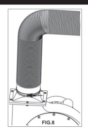
Now fit a hose clamp over the hose and slide one end of the hose over the outlet adaptor; fit the 2nd hose clamp over the other end of the hose and slide that end over the opening in the collector. FIG. 8.
