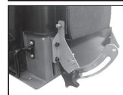
Locate the angle guide and knob and attach to one side of the sander; Repeat steps for the 2nd guide - Please note that one angle guide will be facing inwards).
