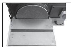
Fix table to table brackets using the 4 bolts supplied.
