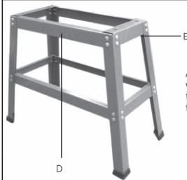
Attach the upper supports (length & width) (D & E) to the frame and complete the leg-set by pressing 4 rubber feet to the bottom of each leg.
