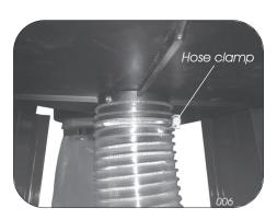
Attach the collection hose to the lower part of the filtration housing and secure in place with the hose clamp (006).
