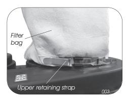
• Slide the upper retaining strap through the bottom of the filter bag, and secure onto the filtration housing (003).
