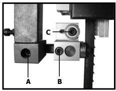
**Allen bolt A -** This allows the bearing assembly support pole to be moved and should be utilised when large movement is required.
