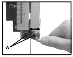
The rear thrust bearings should be set so that they are approximately 3 mm behind the blade. They will only come into contact with the blade as the work-piece is being cut. Due to the many different sizes of band-saw blades available, the rear support bearing needs to have extra movement compared to the lateral support bearings. This is achieved by having 3 different points of movement as opposed to 1 on the lateral support bearings.
